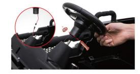
Due to the reason of movement of steering tube, sometimes there is possibility that the hole on the steering wheel and the hole on the steering tube can not match well. If this happens, please use one hand to hold the hook under the car body in order to fix the steering tube. (Referring to the picture)
