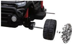
Please take out sleeves from the screw&bolts bags and put into inner and outer sides of front wheels, as well as outer sides of back wheels, and then put one metal gasket into the axle, and then put wheel into the axle, insert the cotter pins to the hole on the axle, and then make the cotter pin across(refer to the photo). Finally, please put the cover onto the wheels.
