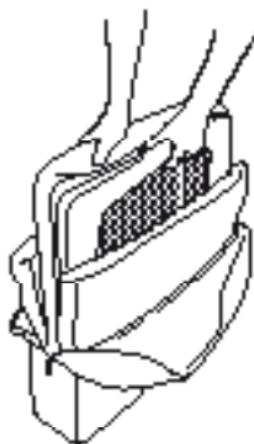
2. Hold the two short sides. Turn the cot so its legs are towards the floor and unfold it with one clear movement so that the legs unfold.
