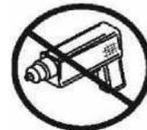
We do not recommend the use of power drills/drivers for inserting screws, as this could damage the unit. Only use hand screwdrivers.
