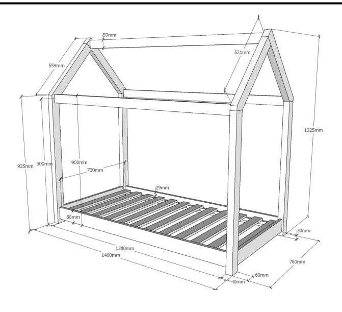
L:1460mm H:1325mm D:780mm 12 Slats 60x12mm plywood
