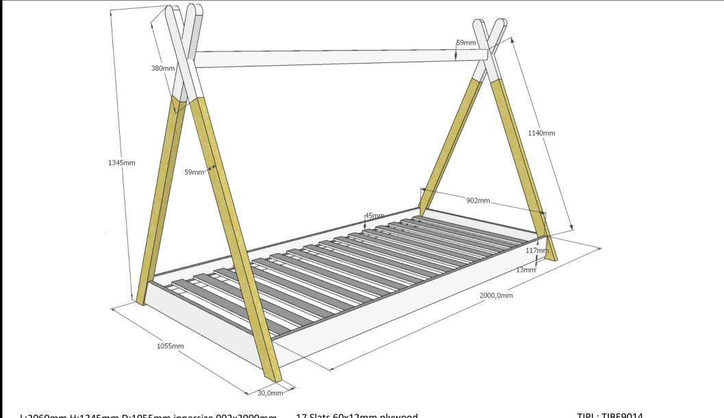
L:2060mm H:1345mm D:1055mm innersize 902x2000mm
